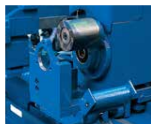
Bending arm can be uplifted for easy replacement of power point rollers
