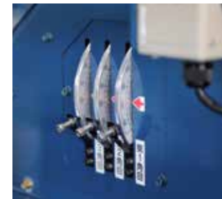
Bending angle setting dial
