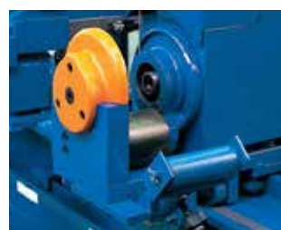
Bending arm can be uplifted for easy replacement of power point rollers
