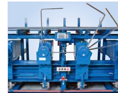
Bending closed hoop
