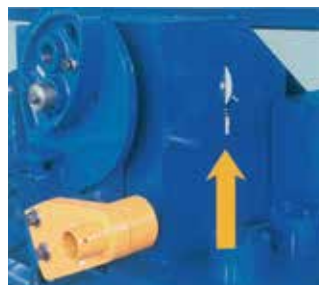
Bending angles setting dial
